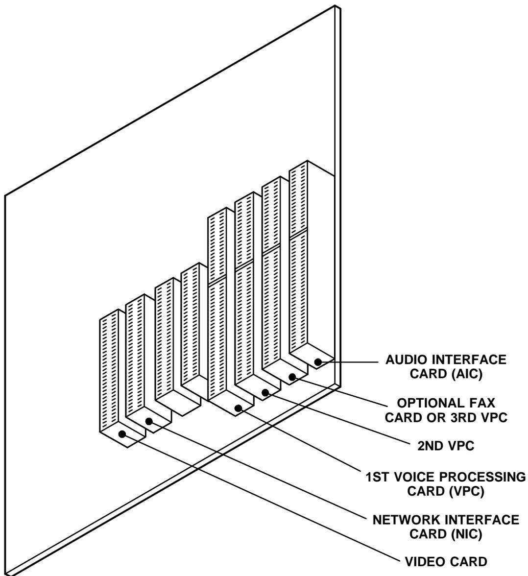
**NOTE:** Depending on the specific model of PC Motherboard being used, the sample card slot arrangement shown above could vary somewhat.
