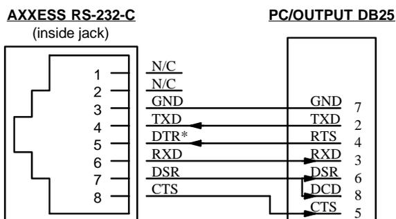
\* The CPU Card RS-232-C port does not support DTR. All other RS-232-C ports (MEM and CPU020/PCM) do support DTR. DB25 internal jumpers: 6-8.
