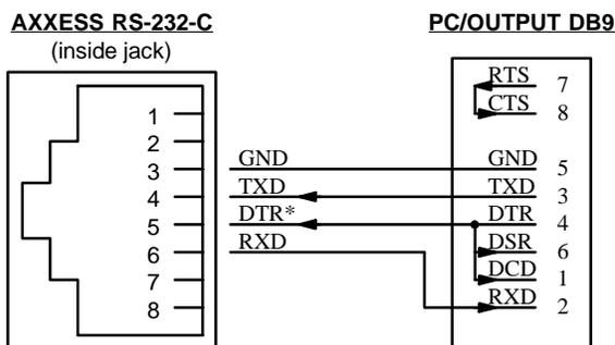
\* The CPU Card RS-232-C port does not support DTR. All other RS-232-C ports (MEM and CPU020/PCM) do support DTR. DB9 internal jumpers: 7-8 and 4-6-1.
