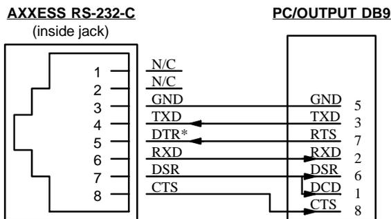
\* The CPU Card RS-232-C port does not support DTR. All other RS-232-C ports (MEM and CPU020/PCM) do support DTR. DB9 internal jumpers: 6-1.
