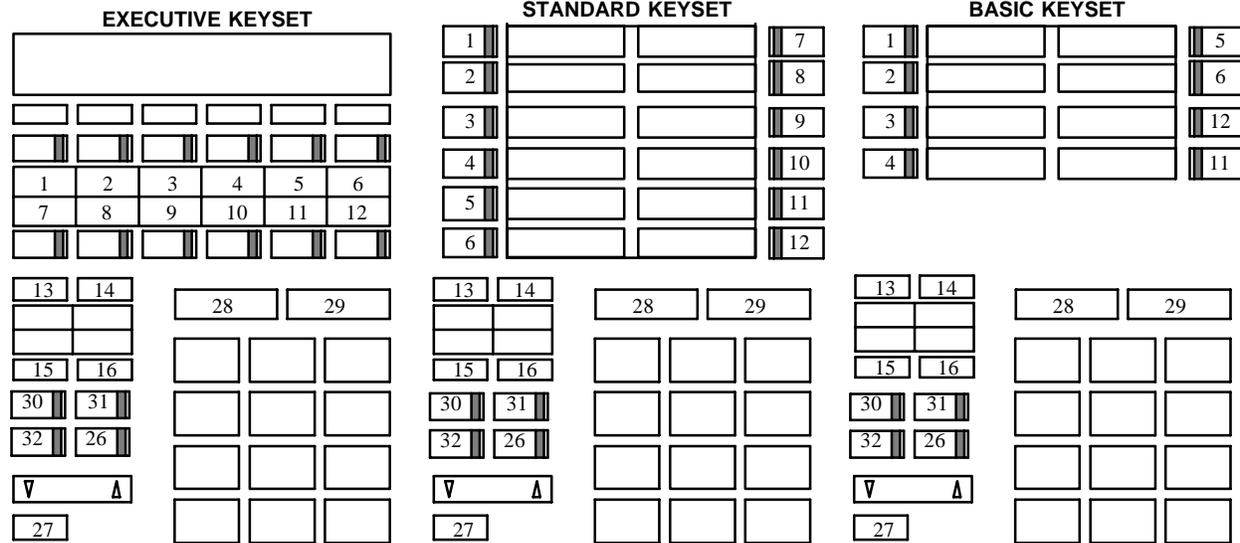
The keys are numbered to show the functions of the keys on the various maps. (Note that when a key is changed on one map, the corresponding key on any other keyset type in that map is automatically changed to match.) Blank keys are not programmable. The keys are defined as follows in the default key maps shown above:
