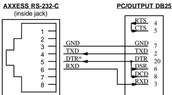
\* The CPU Card RS-232-C port does not support DTR. All other RS-232-C ports (MEM and CPU020/PCM) do support DTR. DB25 internal jumpers: 4-5 and 20-6-8.
