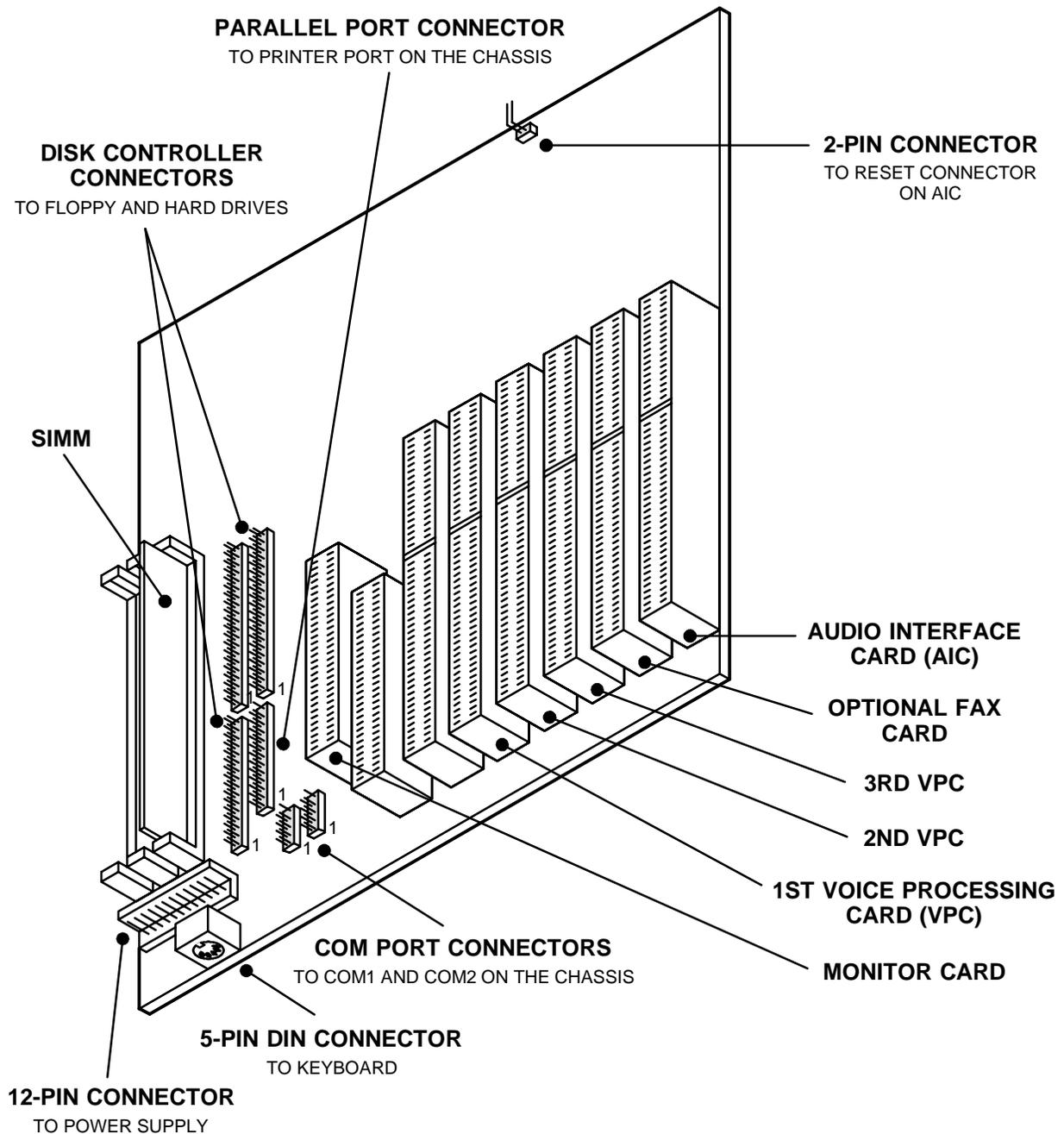
**NOTE:** Depending on the model of PC Motherboard being used, the sample card slot arrangement and the location of the reset connector shown above could vary somewhat.
