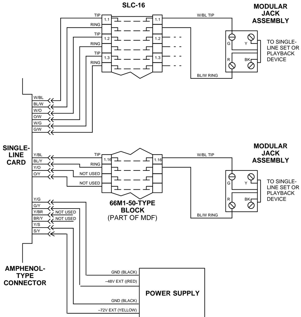
**NOTE:** For simplicity, this figure shows single-line sets and playback devices being installed using one-pair cable and four-conductor modular jacks. Of course, if three-pair cable and six-conductor modular jacks are used instead (as is recommended), extra terminal blocks and the use of cross-connect wiring techniques are required.
